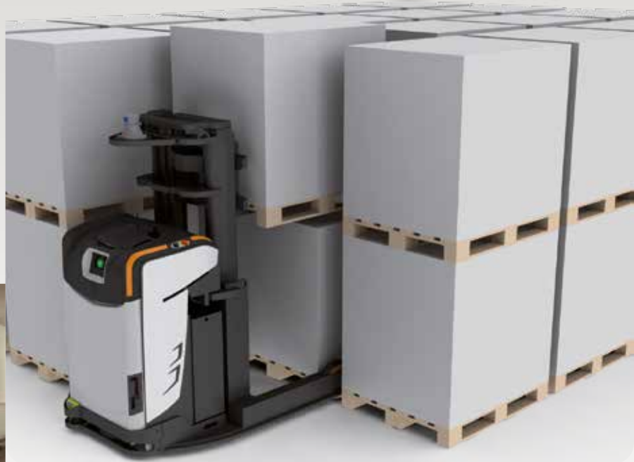
Load-on-load and deep stacking of pallets
