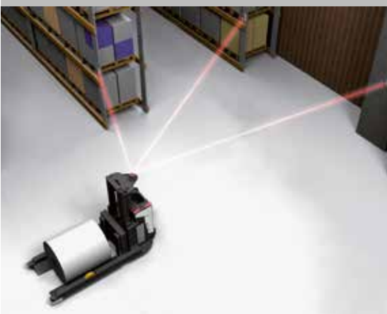
Laser triangulation (the most common)
