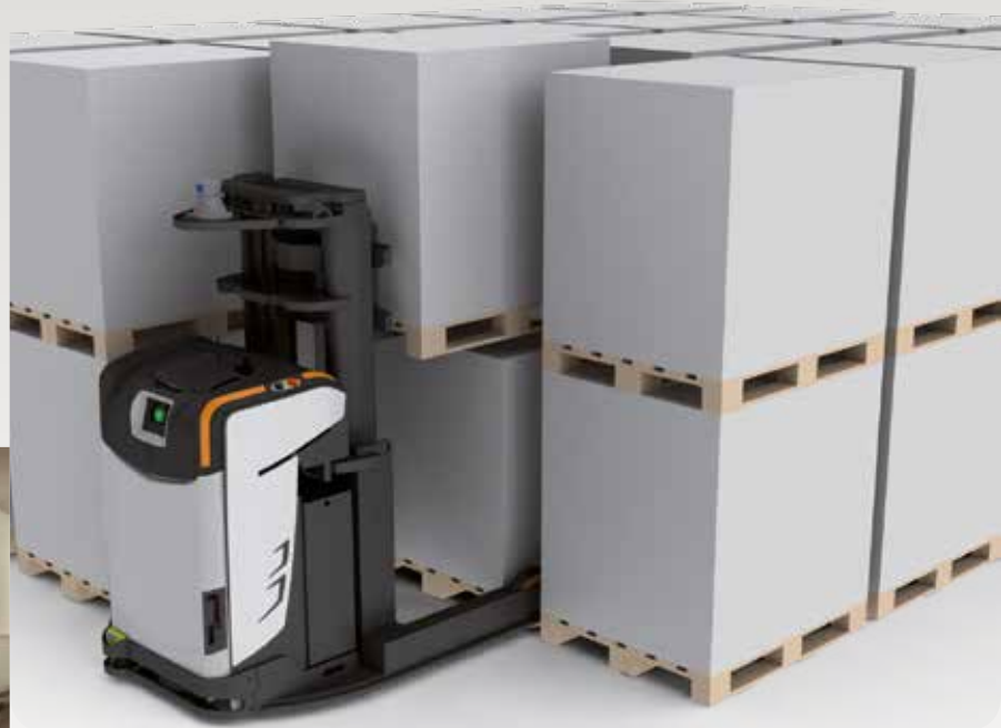
Load-on-load and deep stacking of pallets
